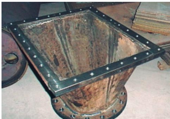
A coal feeding hopper of a power plant.
