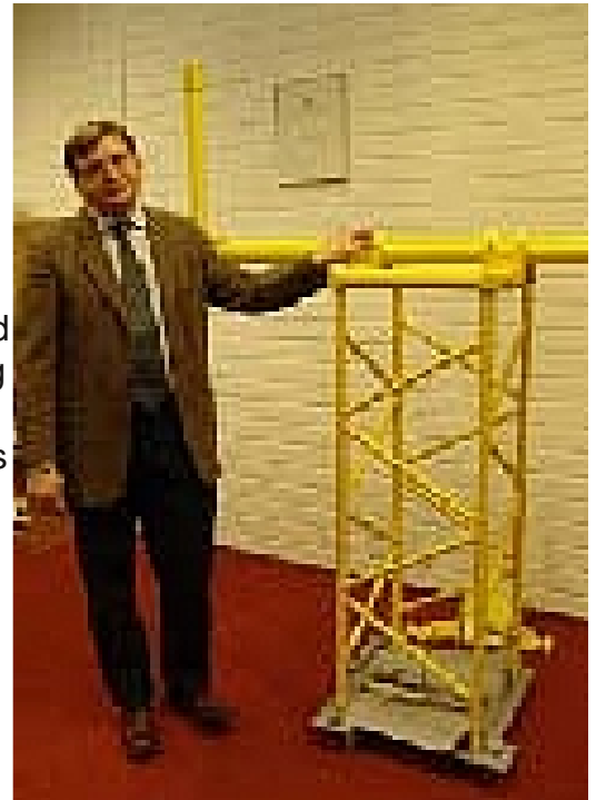
A miniature glass fibre composite top of a lightly constructed airport approach pole. In case of crash a full-size pole goes safely into pieces.
